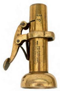
**458.** A SCARCE FIELD'S **PATENT CARTRIDGE TESTER**, the brass body stamped with the manufacturer's details and patent date of 1885. £150-200
